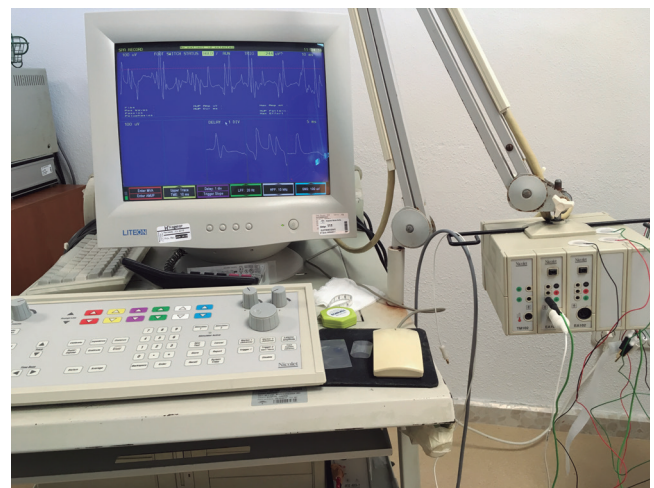
Figure 2. Electromyography equipment and Motor Unit Potential of lateral pterygoid. Biphasic and triphasic morphology waveforms after voluntary muscular contraction can be seen.
